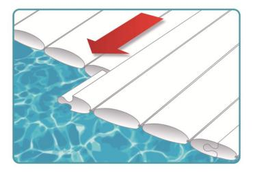
2. At the end of each panel put a screw to fix them together. The screw can be installed on top or below the cover.
